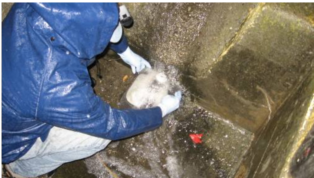
Collecting a sheet flow stormwater sample.
